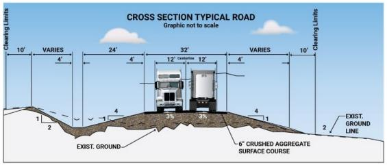
Figure 2-1. Typical roadway section Source: Adapted from DOWL 2016: Appendix 5C Typical Section
