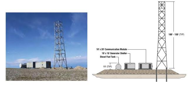
Figure 2-4. Typical communication site layout Source: DOWL 2019
