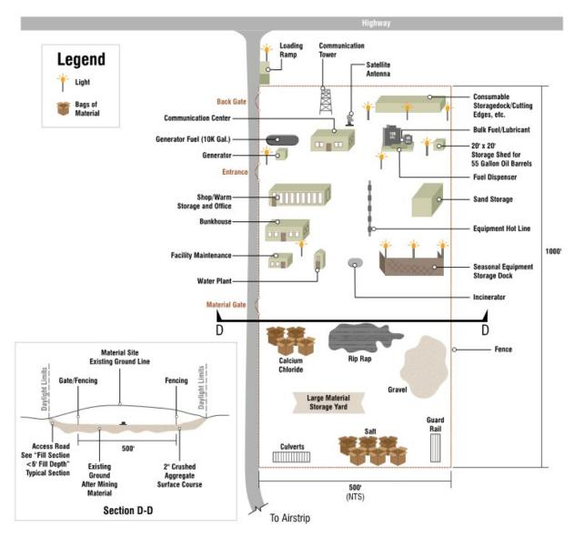
Figure 2-3. Typical maintenance station layout Source: DOWL 2019
