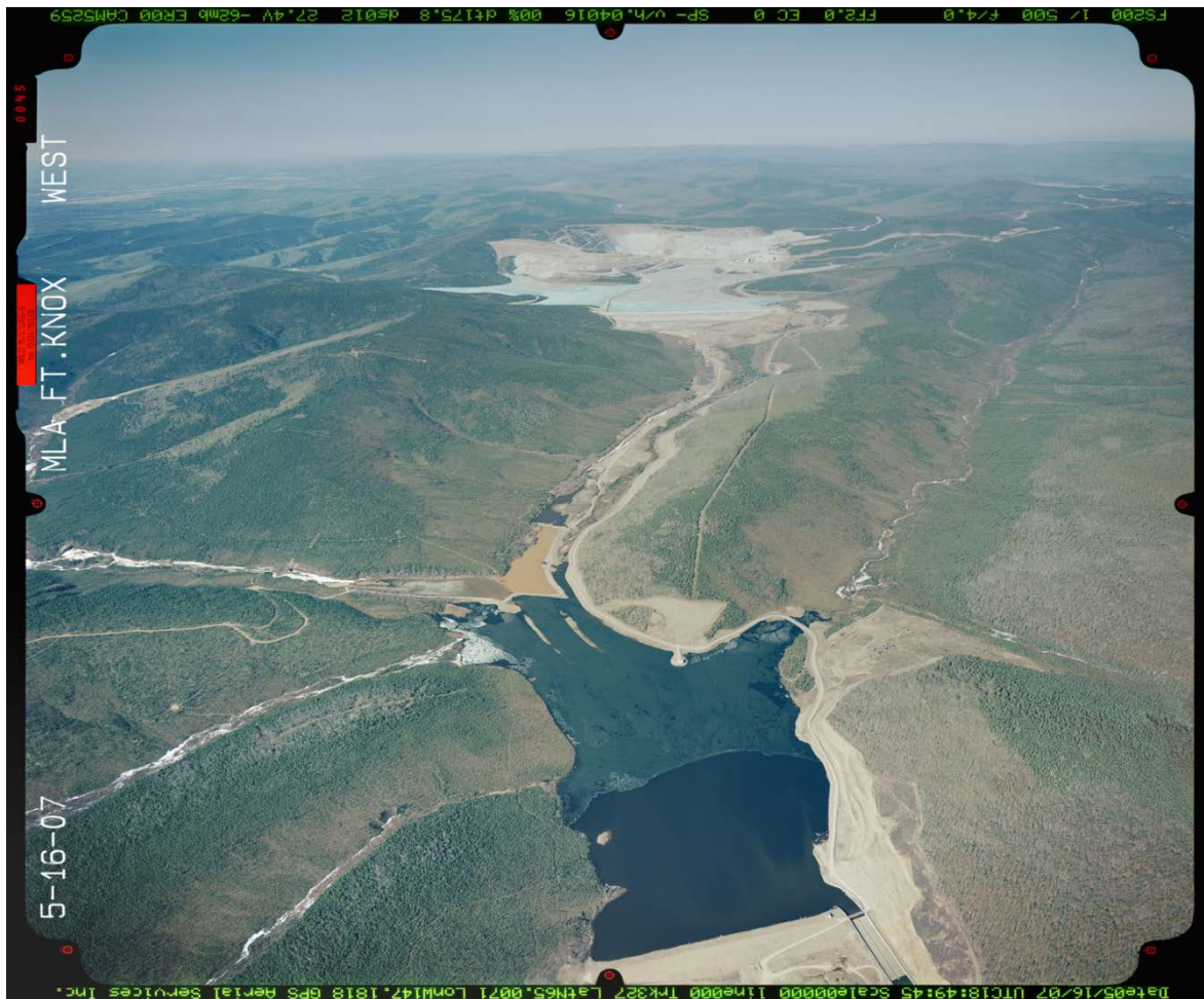
Figure 1. Aerial photograph of the Fort Knox Gold Mine WSR, tailings facility, pit – water supply reservoir in lower part of photo, and the tailings dam and impoundment in the upper Fish Creek valley, photograph provided by FGMI.
