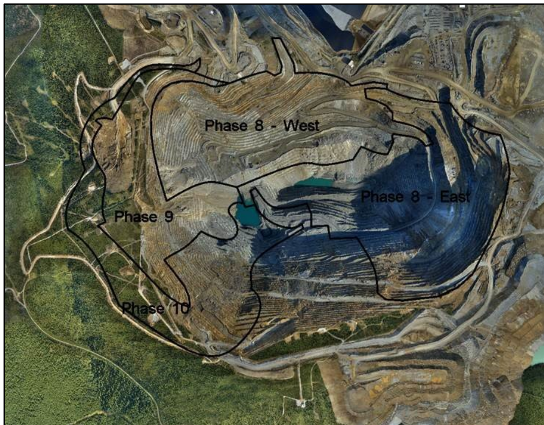
Figure 4: Fort Knox Pit Phases
