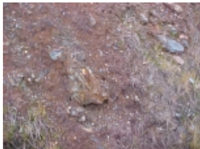
Oxidation of Exposed Pyritic Rock
