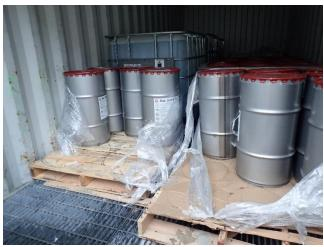
Photo 9. Petroleum products stored within secondary containment.
