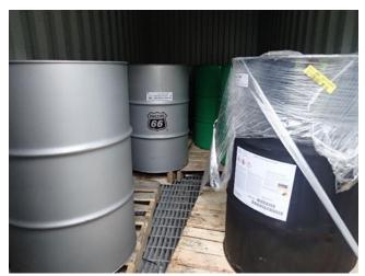
Photo 6. Petroleum products stored within secondary containment.
