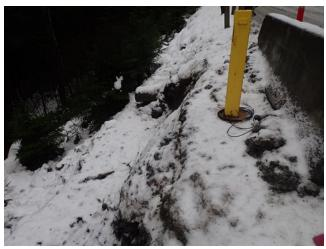
Photo 16. installed inclinometer.
