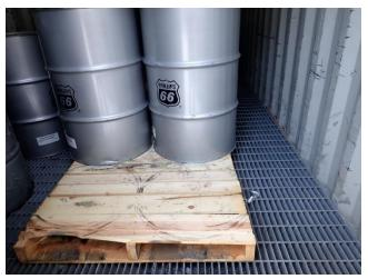
Photo 5. A storage container at the 920 warehouse with secondary containment.
