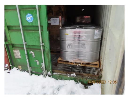
Photo 5. Chemicals stored in appropriate secondary containment at the 920 warehouse area.
