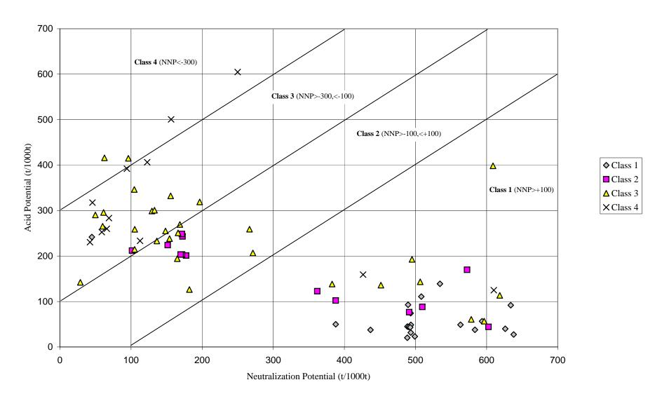
FIGURE 3.27 ACID-BASE ACCOUNTING DATA FOR SURFACE SITE 23
