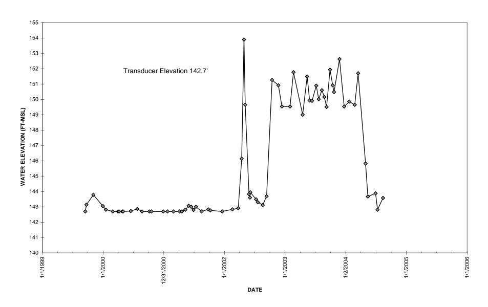
Figure 2.11 Water Level Data for Standpipe Piezometer PZ-T-00-01
