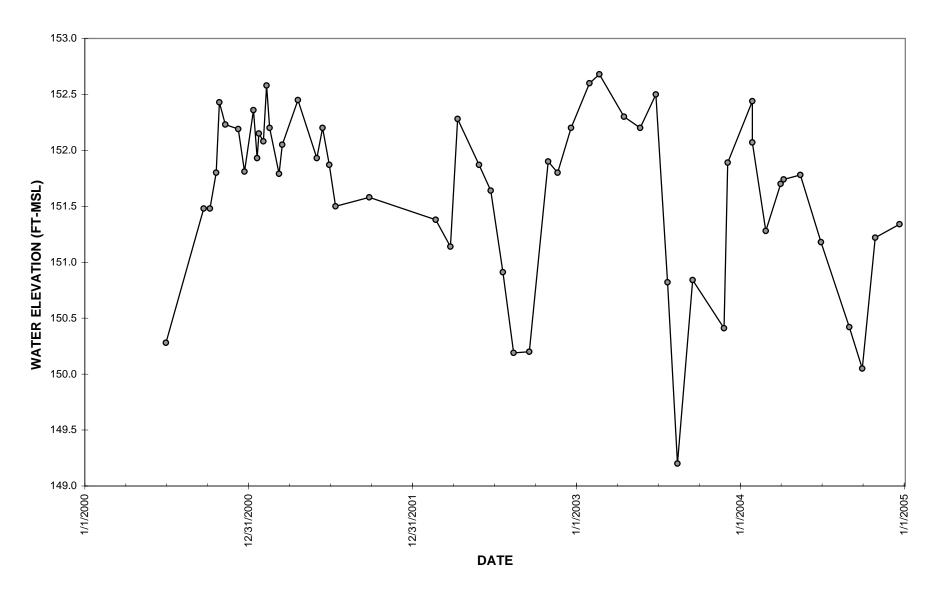
Figure 2.13 Water Level Data for Standpipe Piezometer PZ-T-00-03
