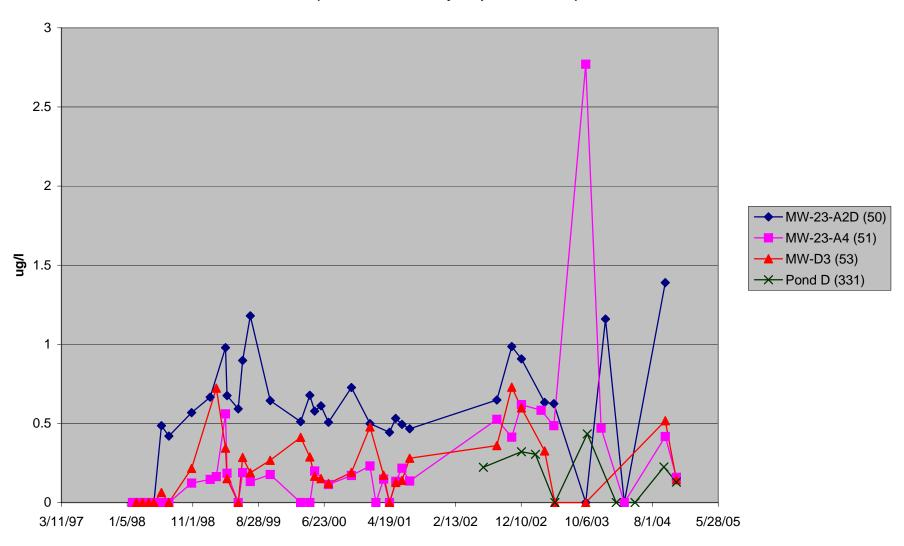
FIGURE 3.20a GREENS CREEK SITE 23/D INTERNAL MONITORING SITES: FINGER DRAINS - ZINC DATA
