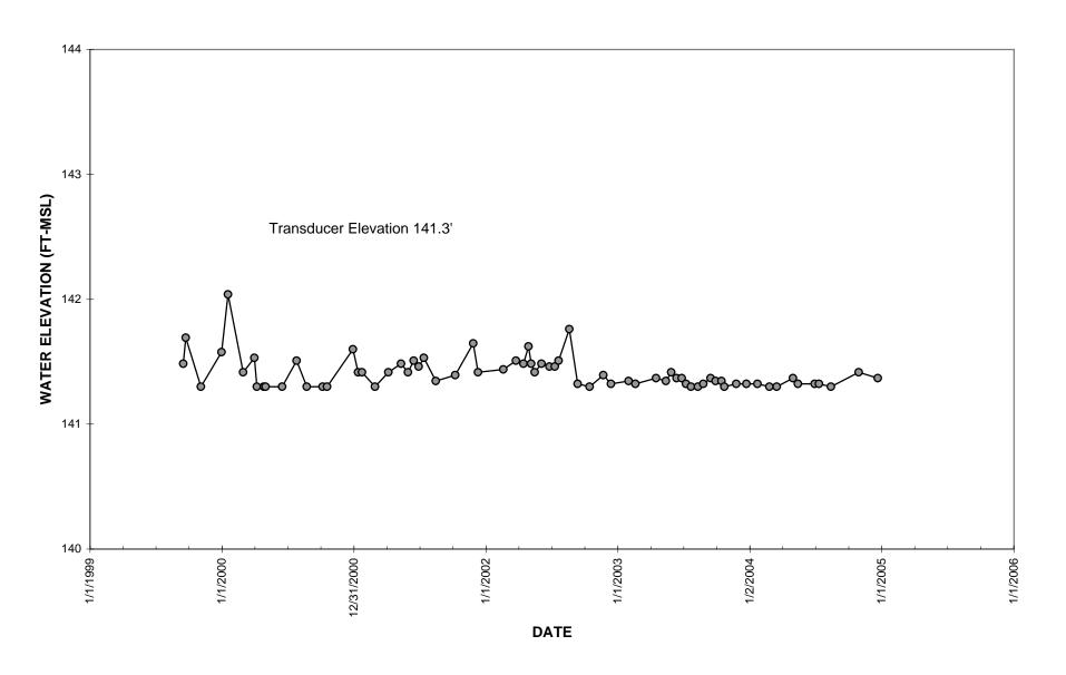
Figure 2.10 Water Level Data for Piezometer 76
