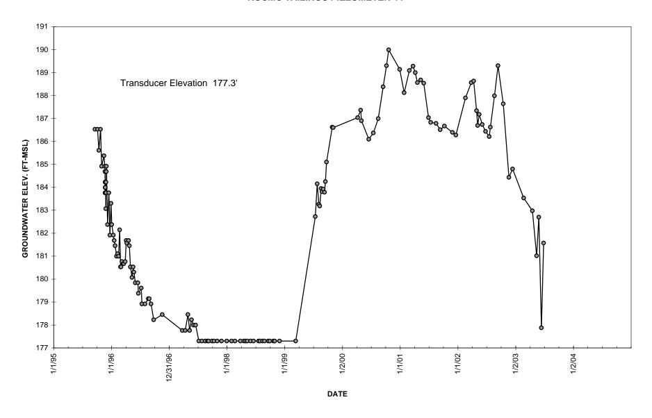
Figure 2.4 Water Level Data for Piezometer 46
