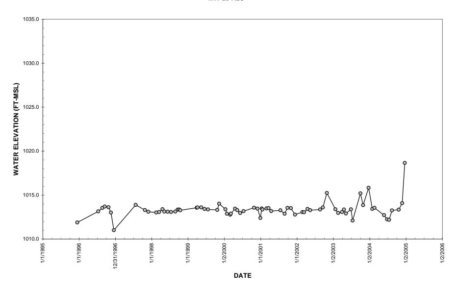
Figure 3.8 Depth to Water Data for Well MW-23-A4
