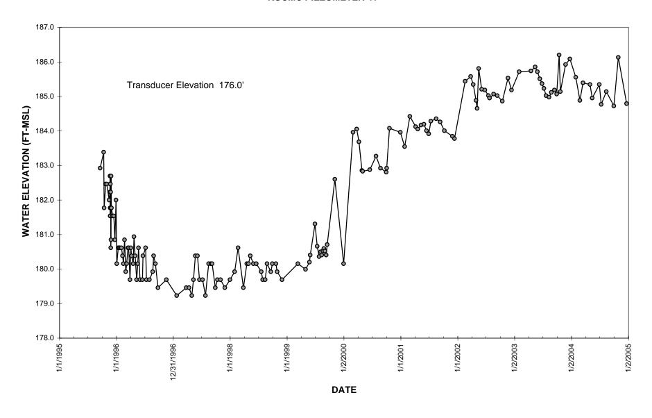
Figure 2.2 Water Level Data for Piezometer 42
