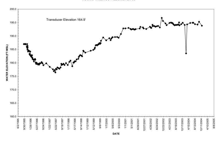
Figure 2.7 Water Level Data for Piezometer 51
