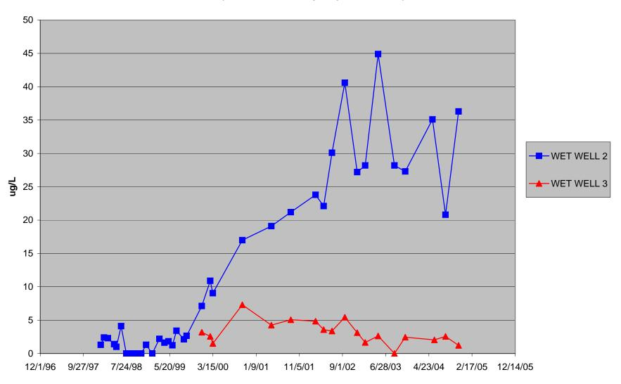
FIGURE 2.25b GREENS CREEK TAILINGS INTERNAL MONITORING SITES: TAILINGS COMPLETIONS - ARSENIC DATA
