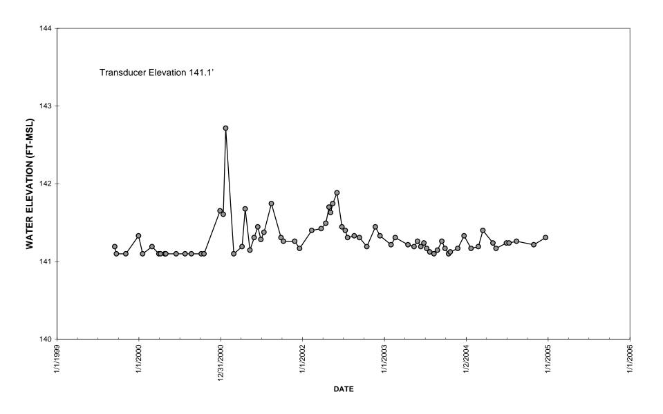
Figure 2.9 Water Level Data for Piezometer 75
