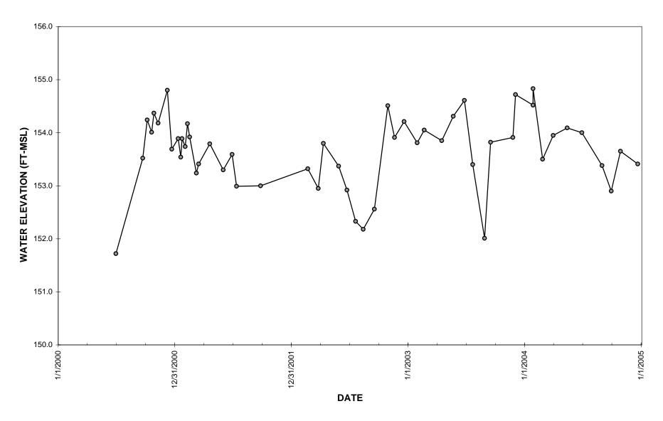
Figure 2.12 Water Level Data for Standpipe Piezometer PZ-T-00-02
