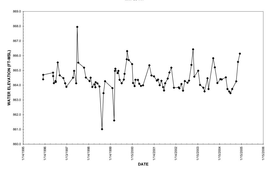
Figure 3.10 Water Level Data for Well MW-23/D-00-01
