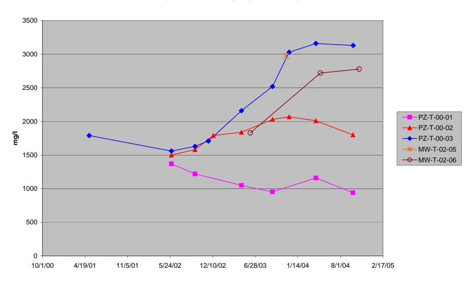
FIGURE 2.24c GREENS CREEK TAILINGS INTERNAL MONITORING SITES: SUCTION LYSIMETERS - SULFATE DATA
