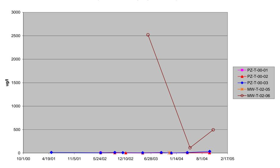
FIGURE 2.26c GREENS CREEK TAILINGS INTERNAL MONITORING SITES: SUCTION LYSIMETERS - ZINC DATA
