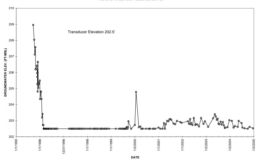
Figure 2.3 Water Level Data for Piezometer 44
