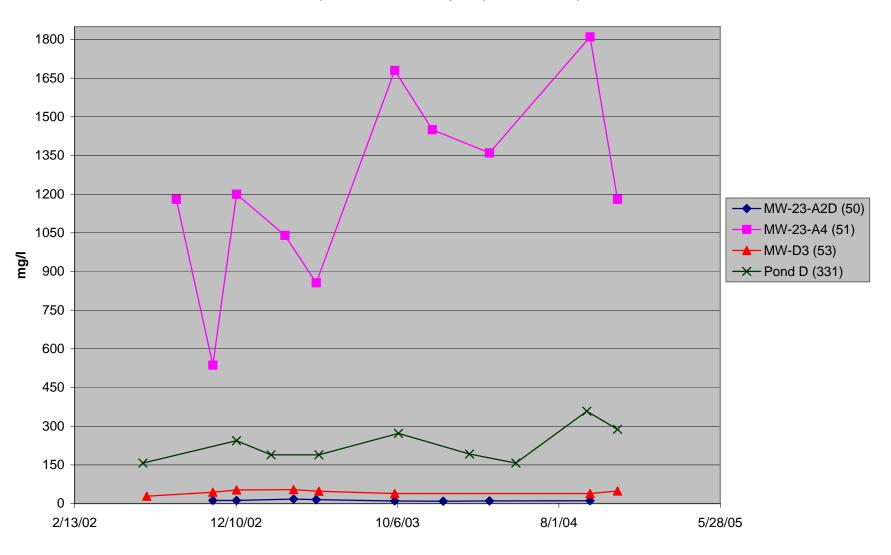
FIGURE 3.19a GREENS CREEK SITE 23/D INTERNAL MONITORING SITES: FINGER DRAINS - ARSENIC DATA
