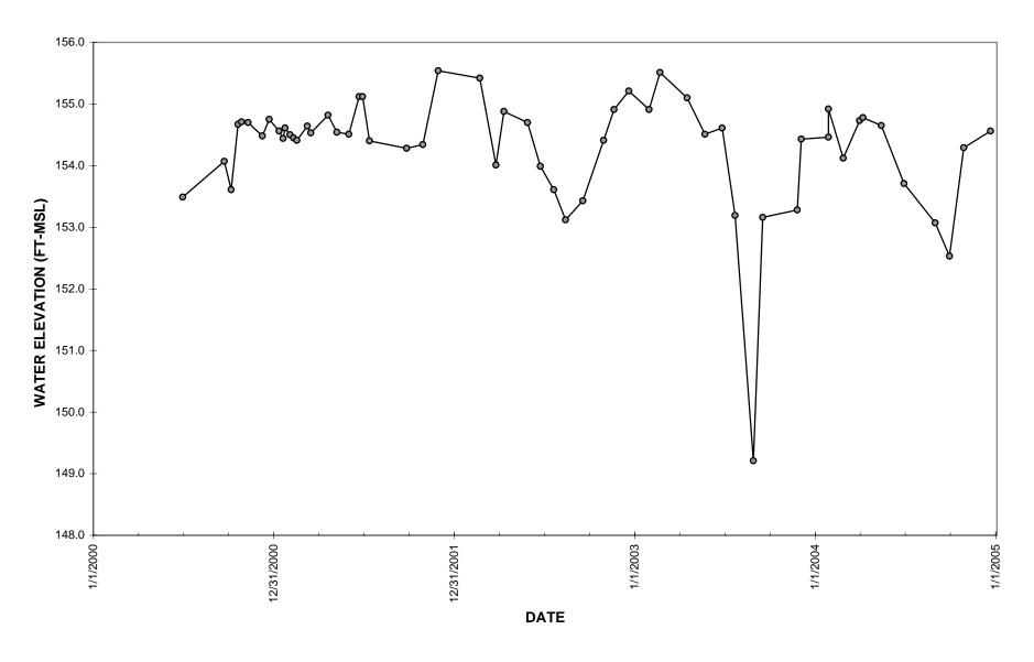
Figure 2.14 Water Level Data for Well MW-T-00-05A
