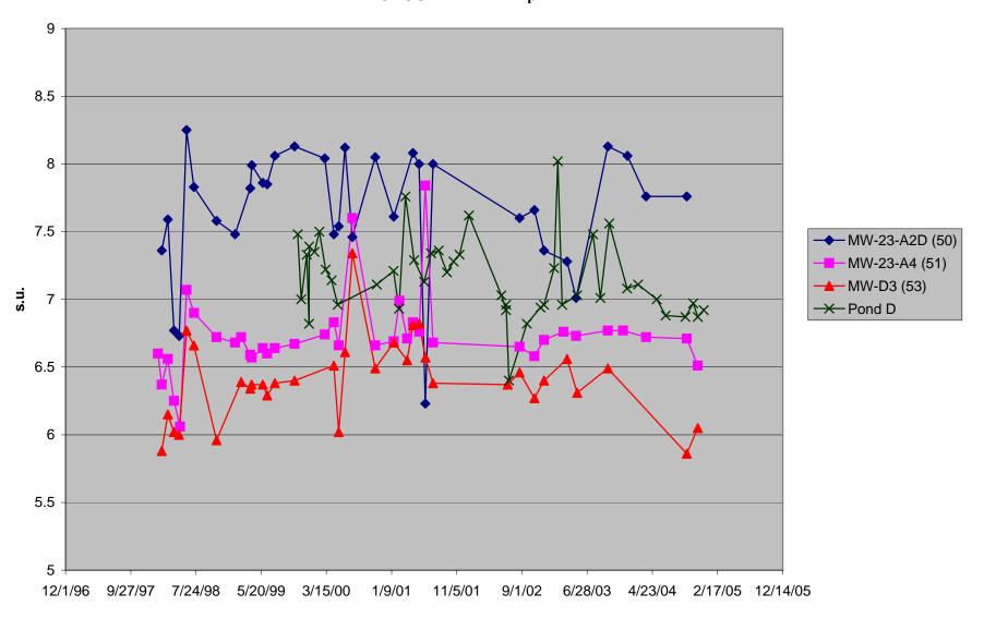
FIGURE 3.15a GREENS CREEK SITE 23/D INTERNAL MONITORING SITES: **FINGER DRAINS - ALKALINITY DATA**
