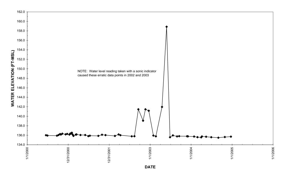
Figure 2.15 Water Level Data for Well MW-T-00-3A
