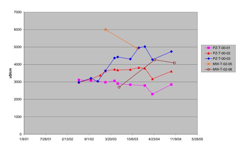
FIGURE 2.22c GREENS CREEK TAILINGS INTERNAL MONITORING SITES: SUCTION LYSIMETERS - CONDUCTIVITY DATA
