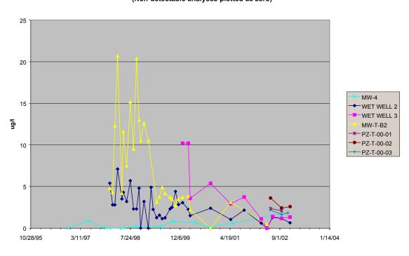
GREENS CREEK TAILINGS INTERNAL MONITORING SITES - COPPER (Non-detectable analyses plotted as zero)
