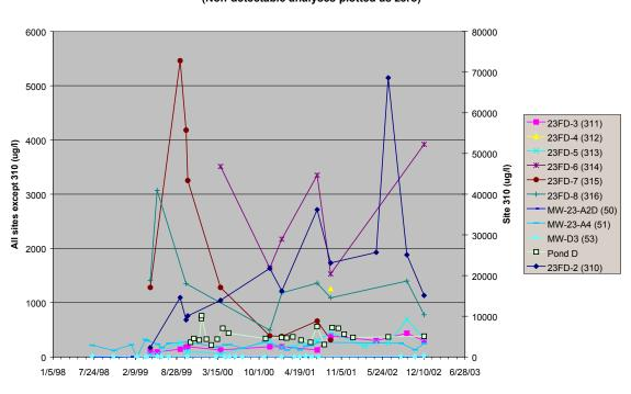
GREENS CREEK SITE 23/D INTERNAL MONITORING SITES - ZINC (Non-detectable analyses plotted as zero)
