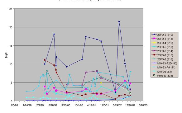
GREENS CREEK SITE 23/D INTERNAL MONITORING SITES - COPPER (Non-detectable analyses plotted as zero)
