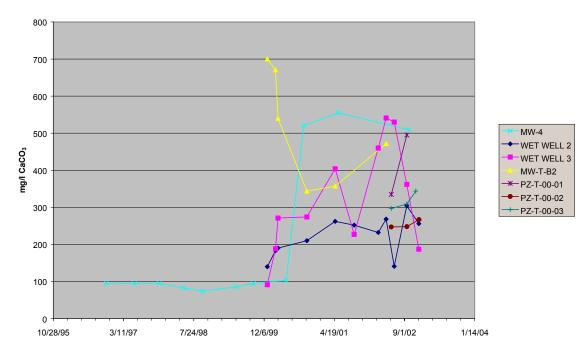
Calcium and magnesium are the primary contributors to hardness (Figure 2.23) and reflect dissolution of carbonate minerals, such as calcite and dolomite. Carbonate dissolution neutralizes acidity formed by sulfide oxidation, which is also the source of sulfate shown in Figure 2.24. Sulfate concentrations range between 500 and 2000 mg/l in the tailings pile waters.
