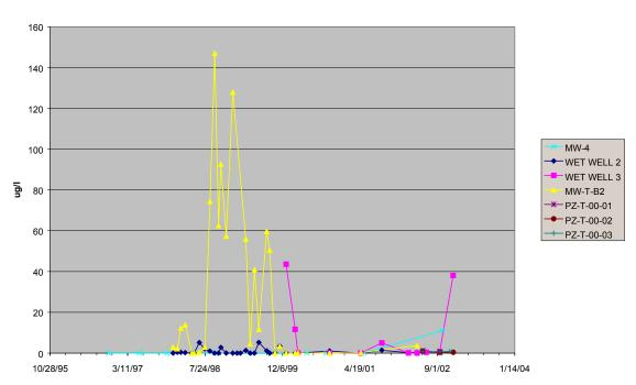
GREENS CREEK TAILINGS INTERNAL MONITORING SITES - LEAD (Non-detectable analyses plotted as zero)
