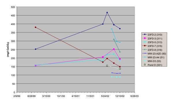
GREENS CREEK SITE 23/D INTERNAL MONITORING SITES - ALKALINITY (Non-detectable analyses plotted as zero)
