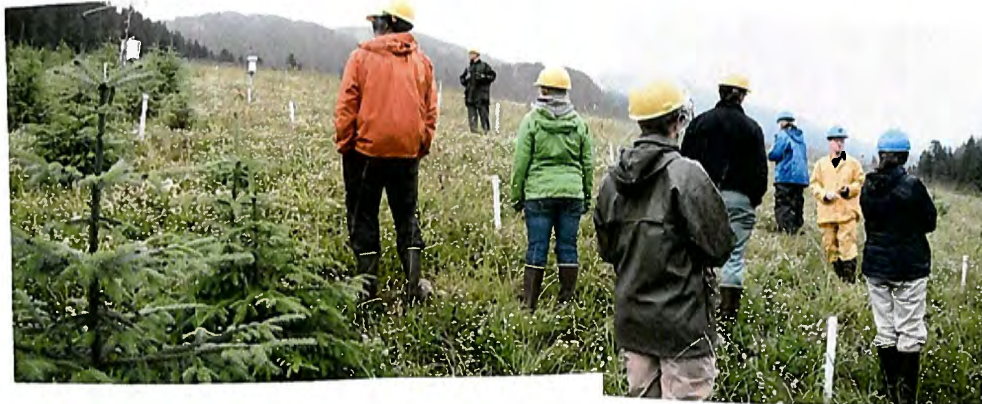
Test Cover System at Site 23. Note volunteer conifer growth and monitoring probes. Also note clover and grass growth on the cap. Deer and bear are excluded by an electric fence that surrounds this test plot
