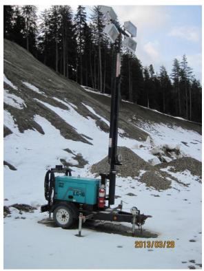
Photo 1. Mobile light plant in 1.4 Mile A Road Pit lacks secondary conatinment.
