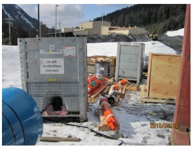
Photo 8. Examples of lack of secondary containment at the warehouse.
