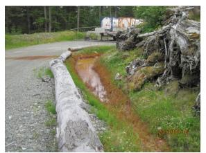
Photo 1a. Reddish-stained water emanating from the waste rock pile with ph of appox 7.
