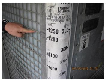
Photo 05. Tote with approximately 330 gallons stored in containment designed for 299 gallons.
