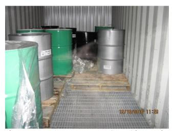
Photo 7. A 920-area storage container with secondary containment.
