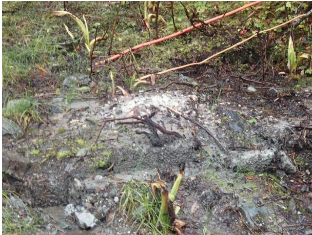
Photo 11. A reclaimed or "plugged" borehole.
