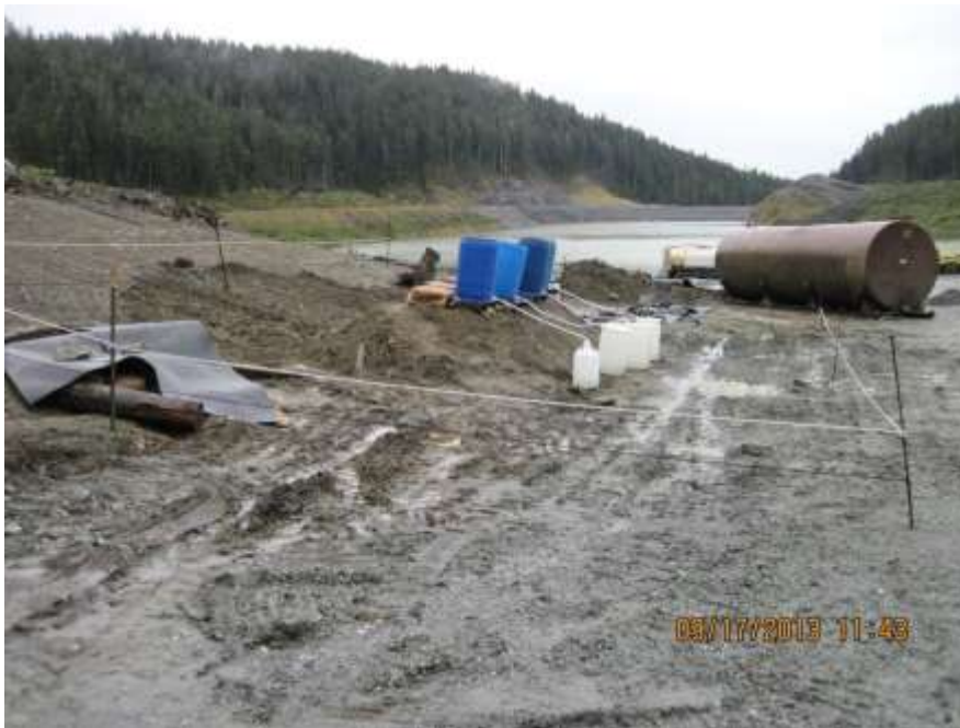
Photo 09. The field test cells have not been secured with a fence as required. It is important that this area not be disturbed for the life of the mine.
