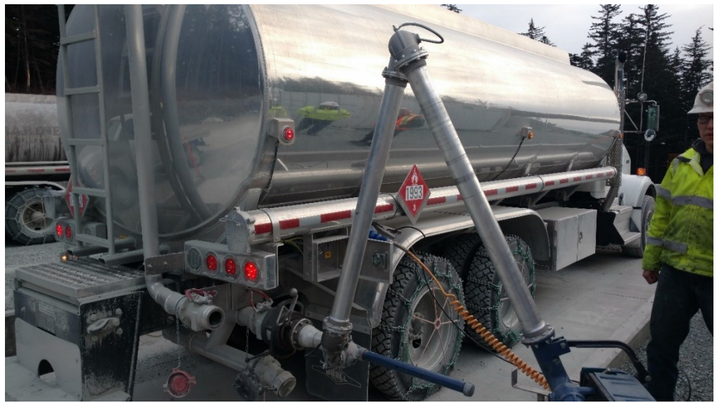
Figure 9 A fuel truck being filled at the tank farm.
