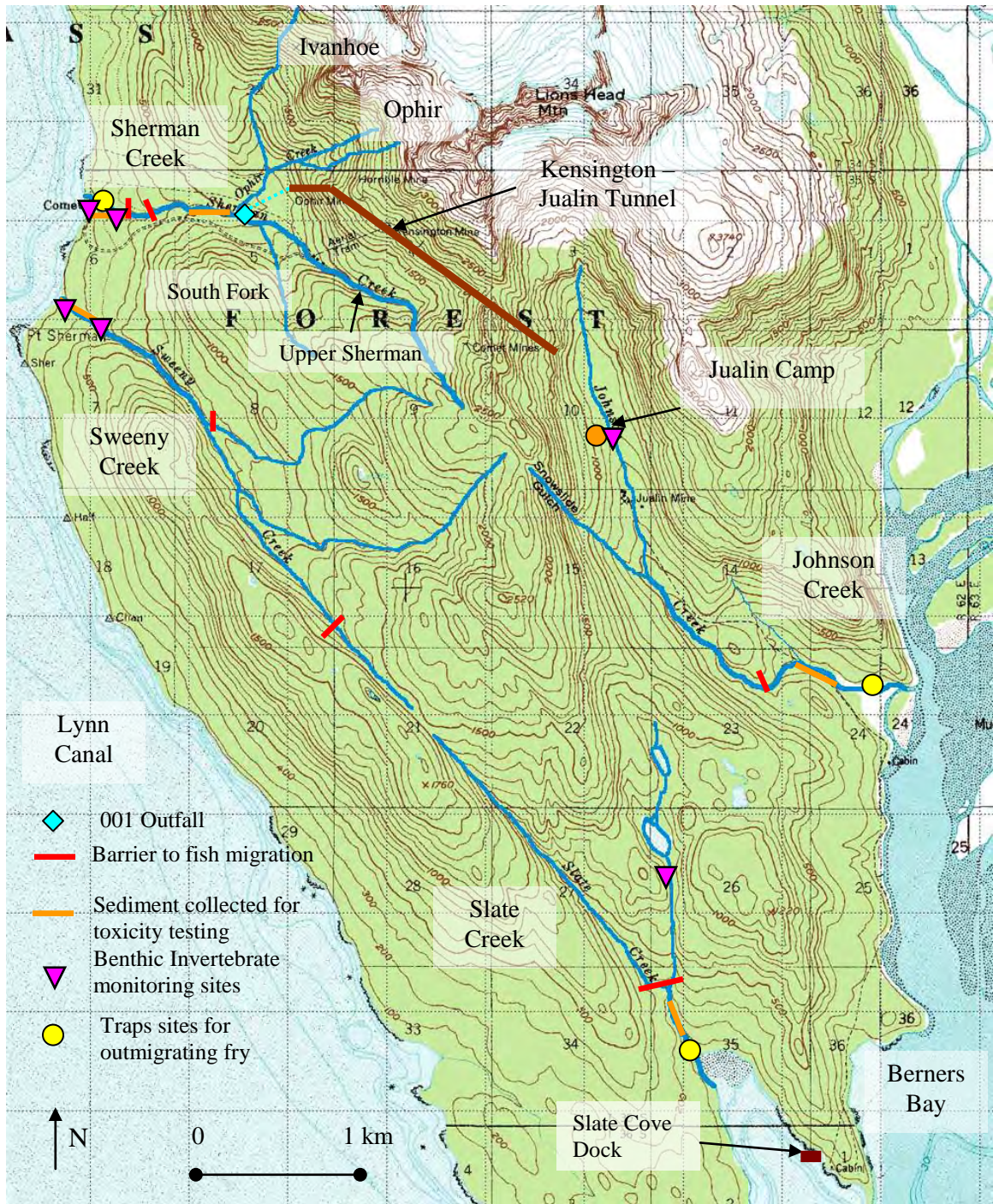
Figure 1: Location of streams near Kensington Mine included in 2010 Aquatic Resource Monitoring. Sediment toxicity testing, benthic invertebrate surveys, resident and anadromous fish surveys, analysis of spawning gravel and aquatic vegetations surveys were conducted in Sherman, Johnson and Slate Creeks. Benthic invertebrates were also collected from two reaches of Sweeny Creek.
