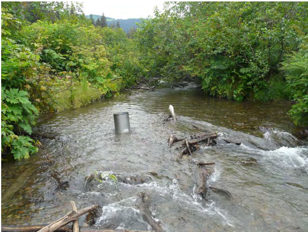
Figure 26: McNeil sampler in place at Reach 2 of Johnson Creek.
