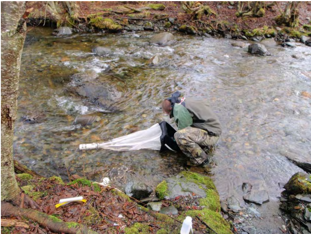
Figure 4: Surber sampling net is being used to gather invertebrates at Sherman.
