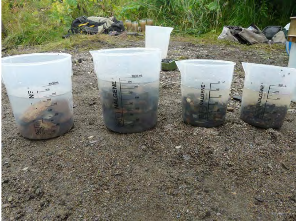
Figure 27: Displacement of water is used to measure volumes of gravel.
