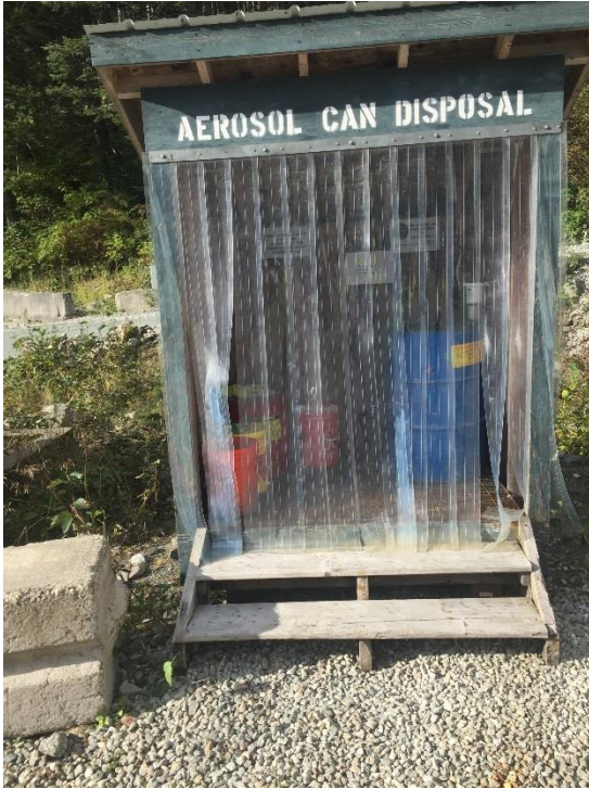
Photo MM showing an aerosol can disposal station, cans are punctured and discharged directly in to a 55 gallon drum containing a Hazardous Waste Label.
