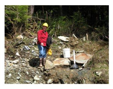
Barry Hogarty at a ground water monitoring well. Cone installed around the pipe to shed surface water so that a better ground water sample can be obtained.
