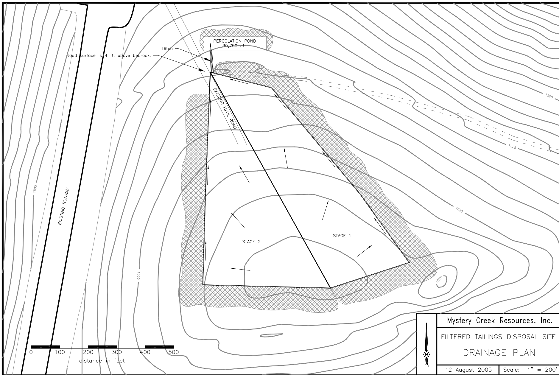
Figure 2.6: FILTERED TAILINGS DISPOSAL SITE DRAINAGE PLAN
