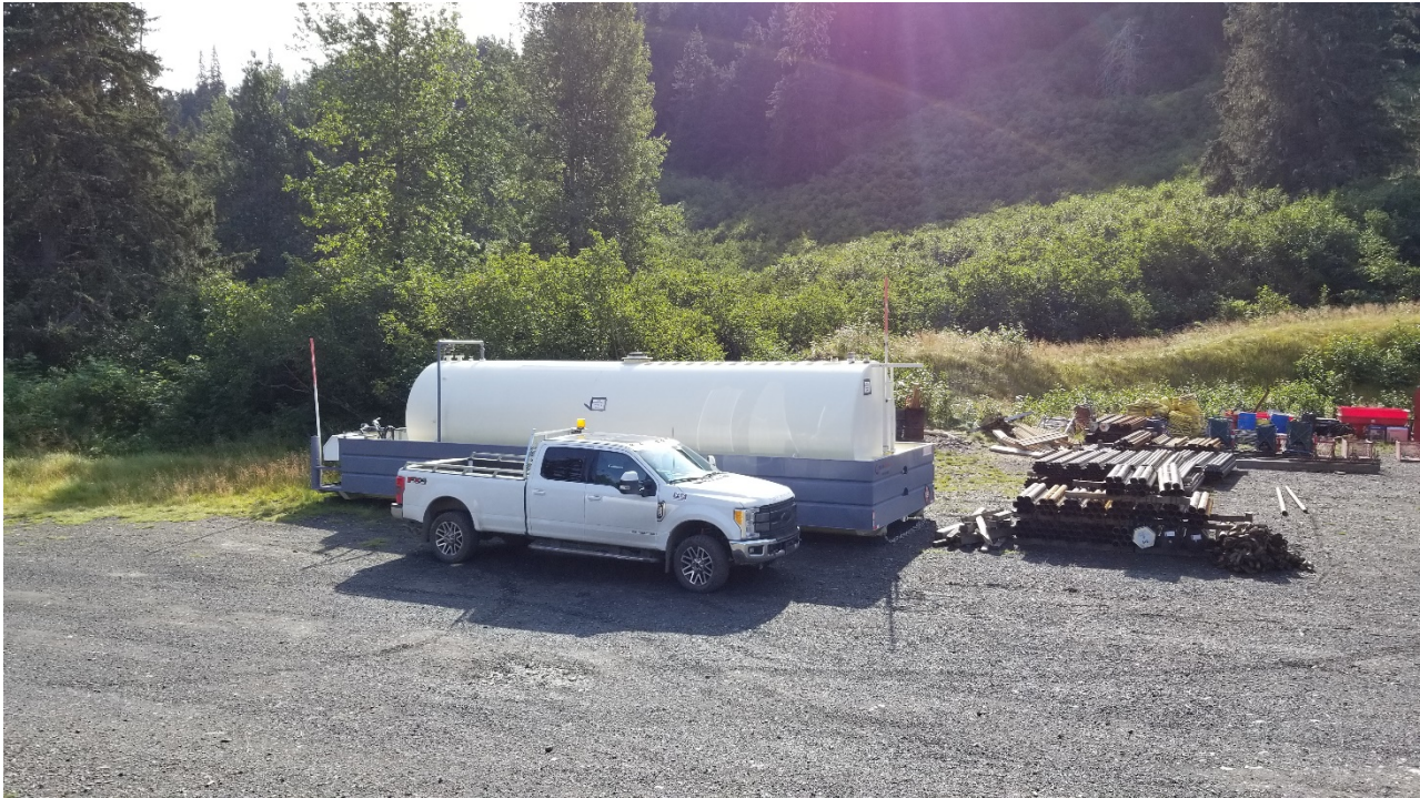
Photo 2. 10,000 gallon fuel tank at Glacier Creek Laydown (added in 2018). Note that this tank is currently not in use and is staged for Phase II Plan of Operation.
