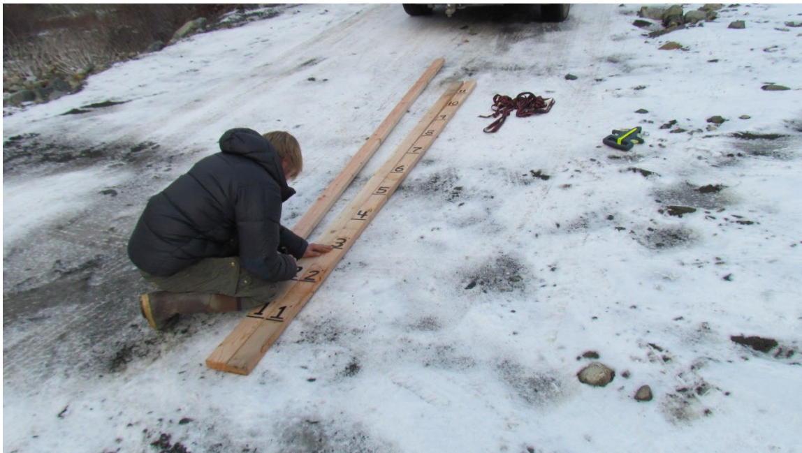
Figure 5. Preparation of staff gauges.
