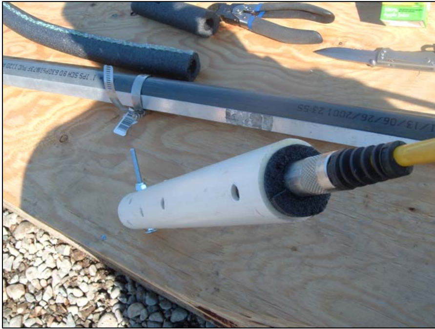
PHOTO 4.1-1: Close-up of datalogger/transducer fixed in stilling-well
