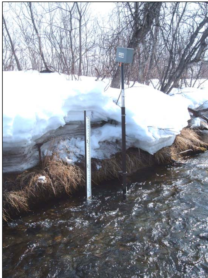
PHOTO 4.1-2: Typical continuous gage and staff gage (installed)
