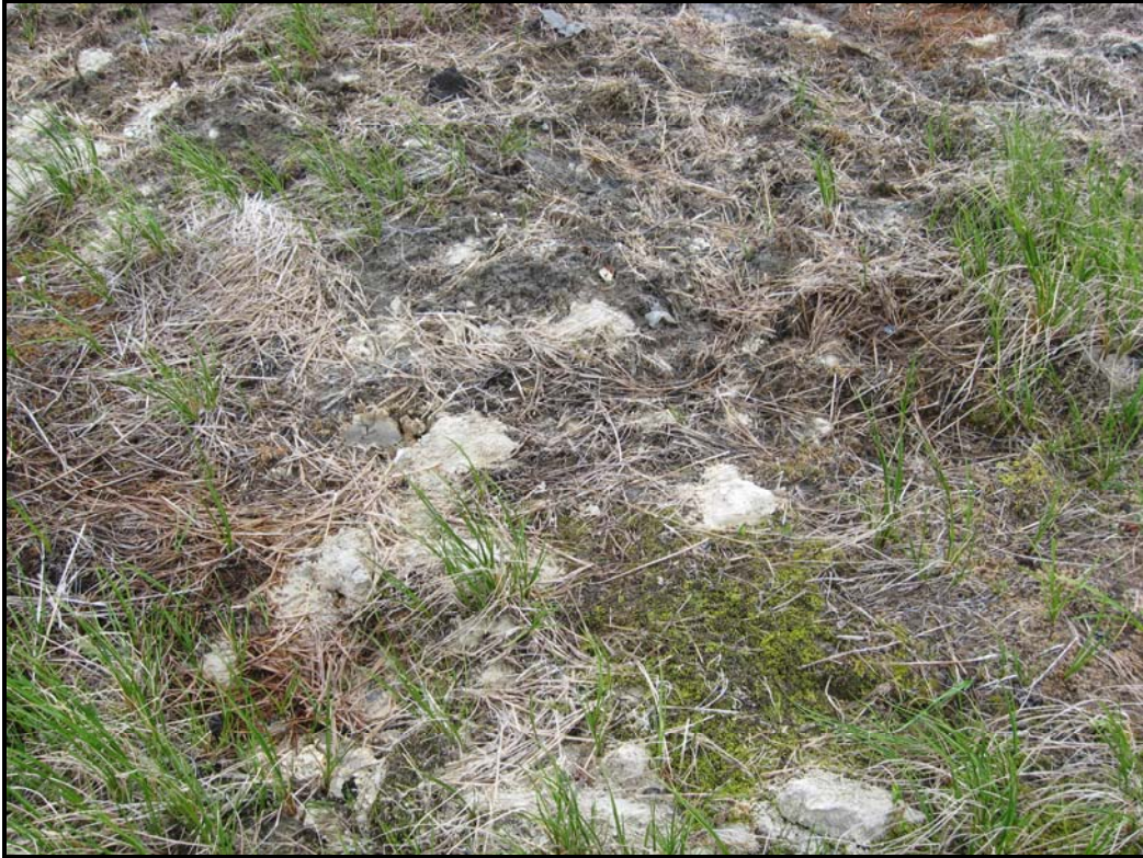
Figure 16. The ground surrounding DH 8412 was not clean and had, what appears to be, clumps of bentonite clay present.
