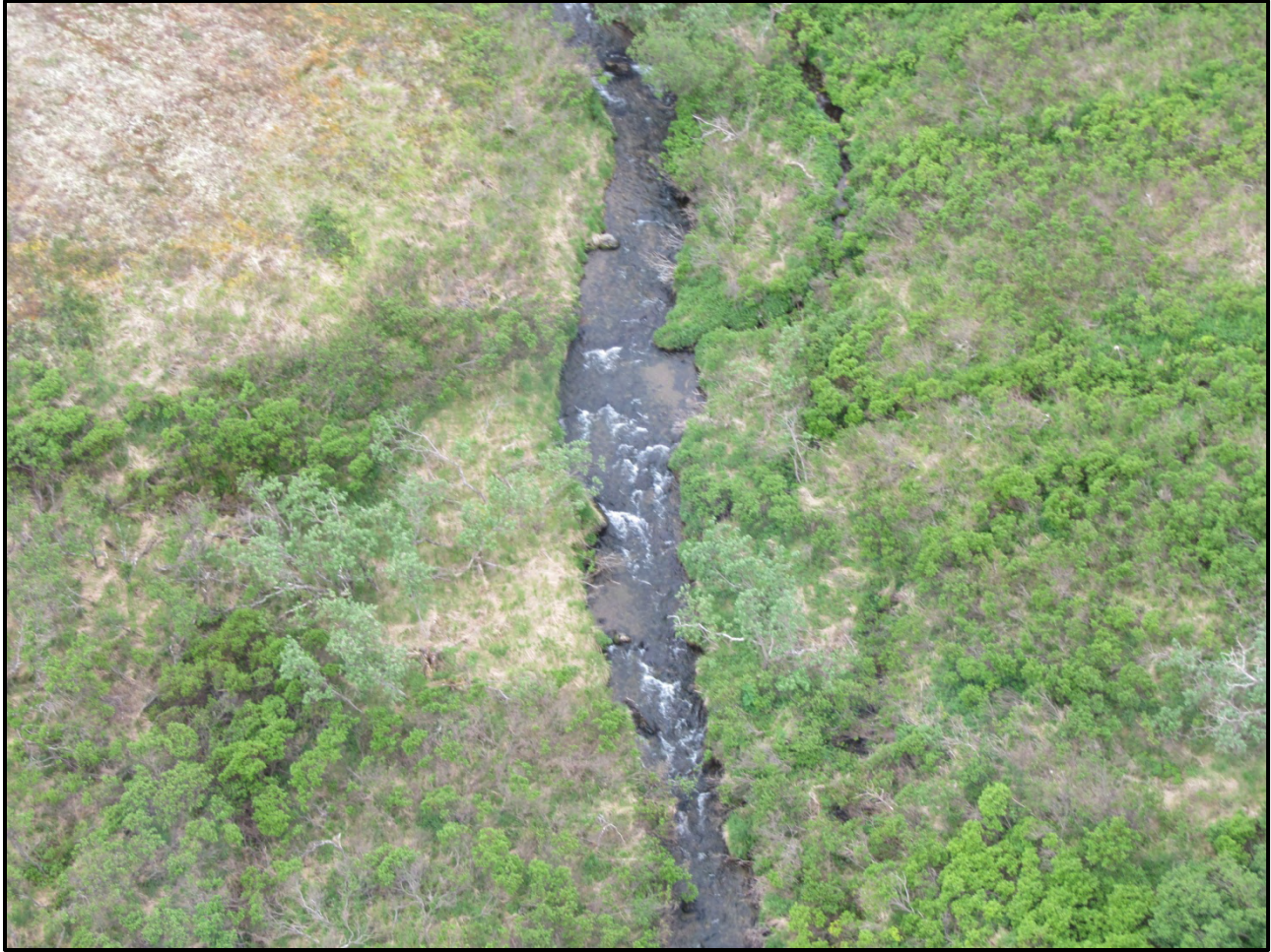
Photo #25. Image displays an example type of channel where streamflows would be calculated/estimated upstream from the withdrawal point (pump) using the float method.
