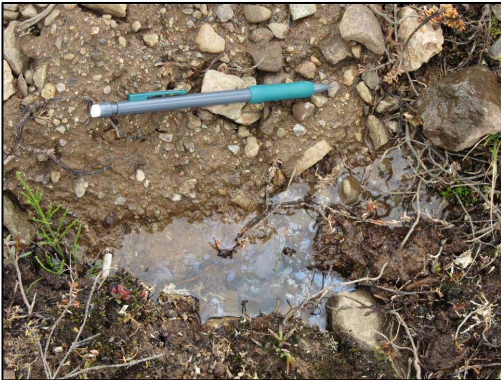
Photo #17. Iron bacteria sheen on water surface. Sheen disseminated when disturbed, which suggests that the source is not from a petroleum product.
