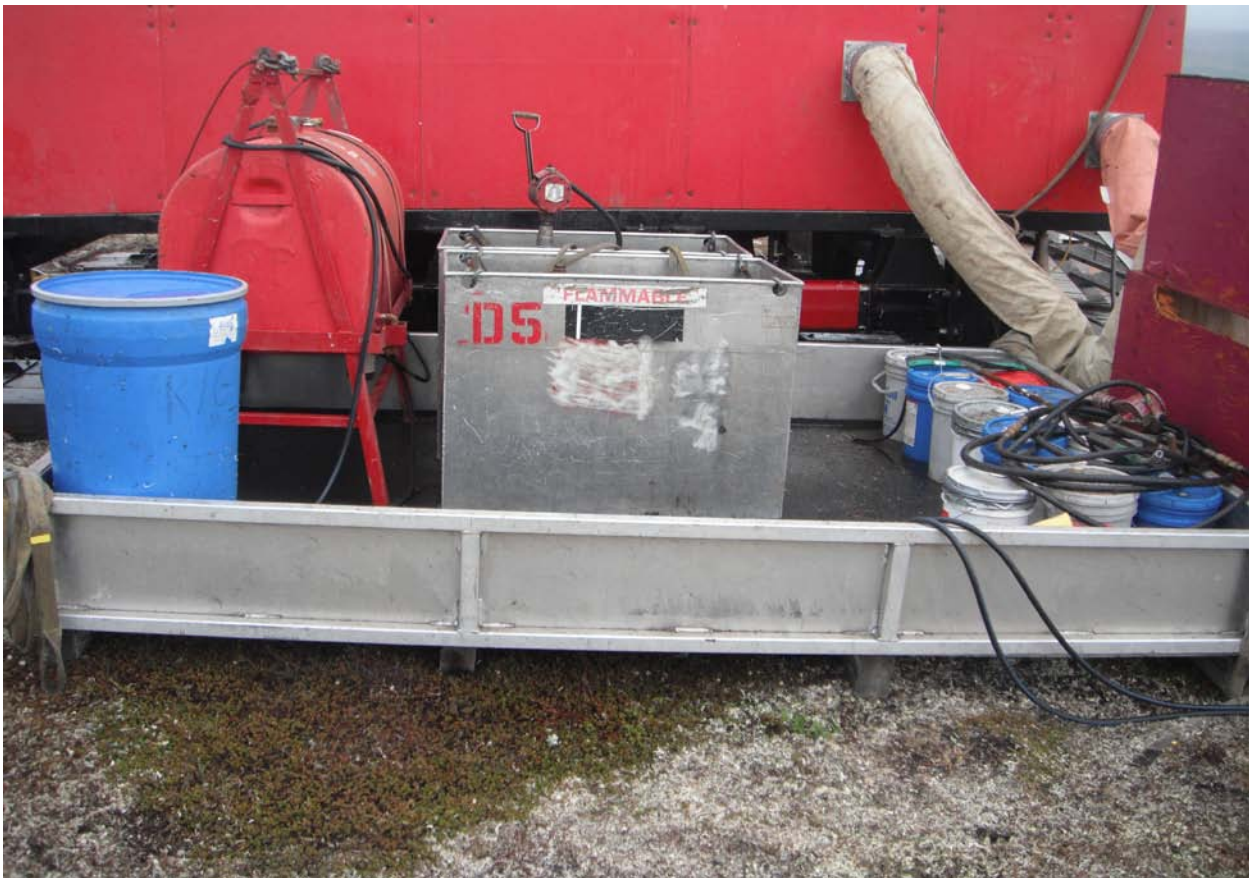
Figure 2 – Drill Hole 11533 Fuel Containment and Spill Kit
