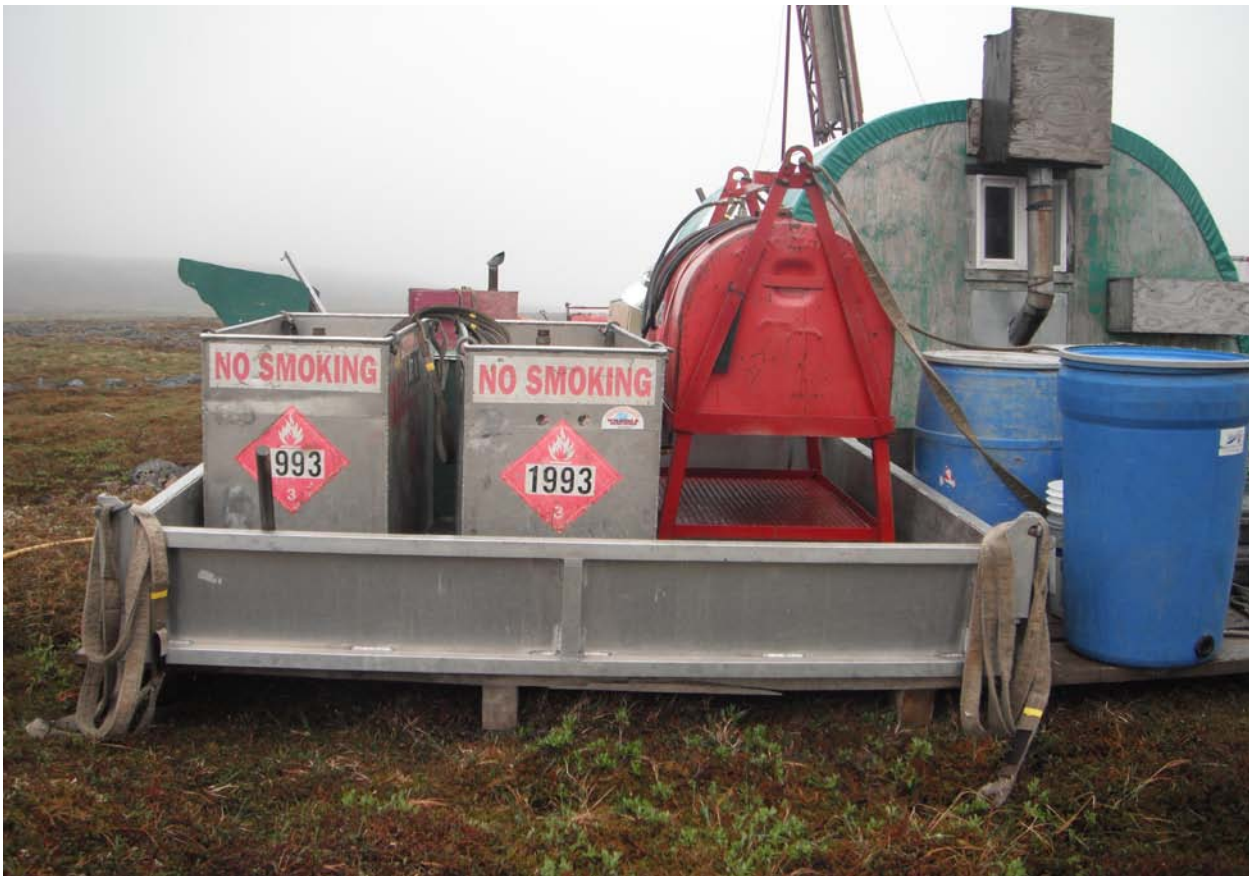
Figure 6 – Drill Hole 11532 Fuel Containment and Spill Kits
