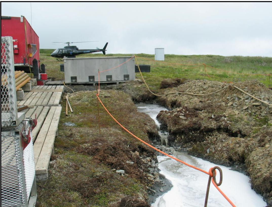
Figure #5. Sump pits and mud recycling tank at DDH 10497 Pebble Field Monitoring Report Cole and O'Donnell
