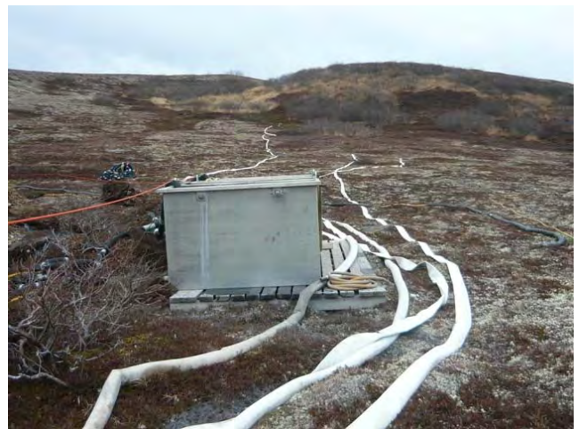
Godwin pump with blue intake & white outlet hoses.
