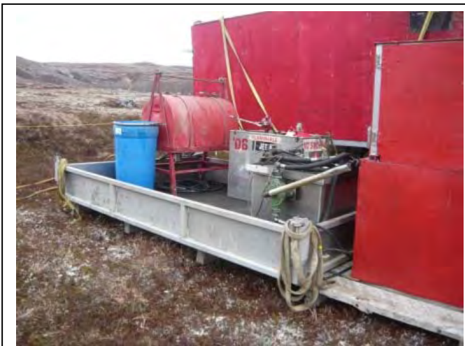
Fuel containment and cleanup kit, next to drill rig #2.
