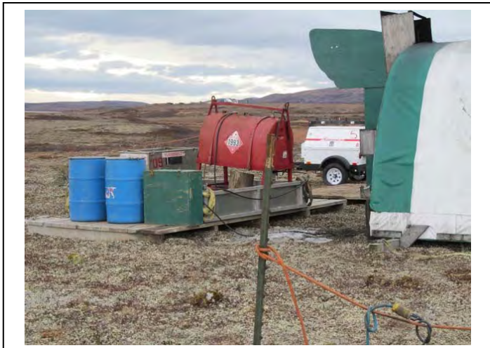
Fuel containment behind driller shack.
