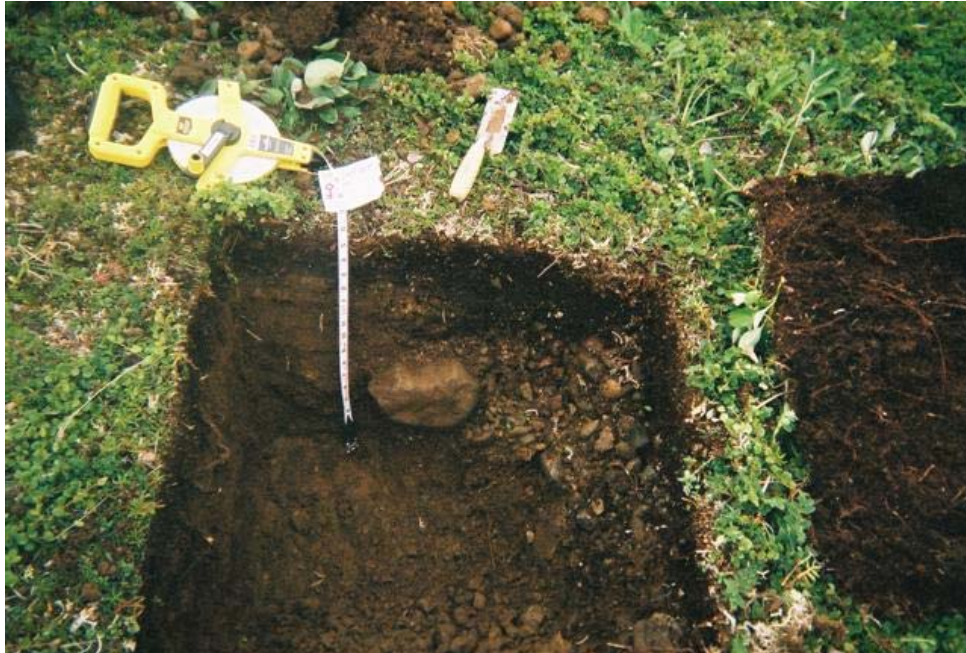
FIGURE 14-41: Test Pit TH-012, showing the typical deposit found along the slopes, where some soil accumulation and formation has occurred.
