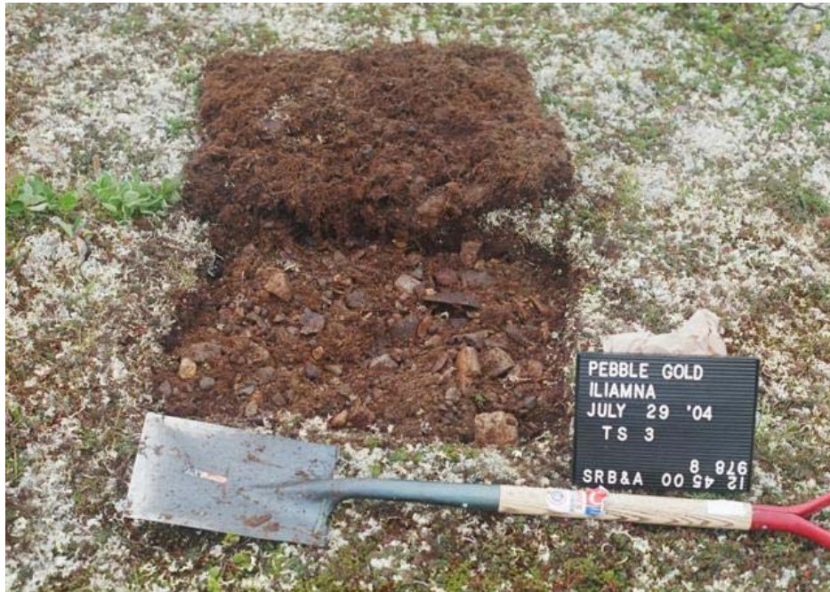
FIGURE 14-44: One of many test pits near the lakes and valley bottoms that showed very thin soil accumulated over beds of frost-shattered gravels and cobbles.
