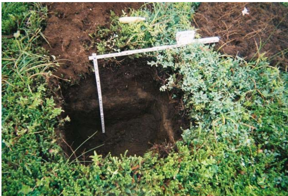
FIGURE 14-42: Test Pit TH-106, one of a few test pits with stratified deposits. Note the grey band, a possible tephra deposit.
