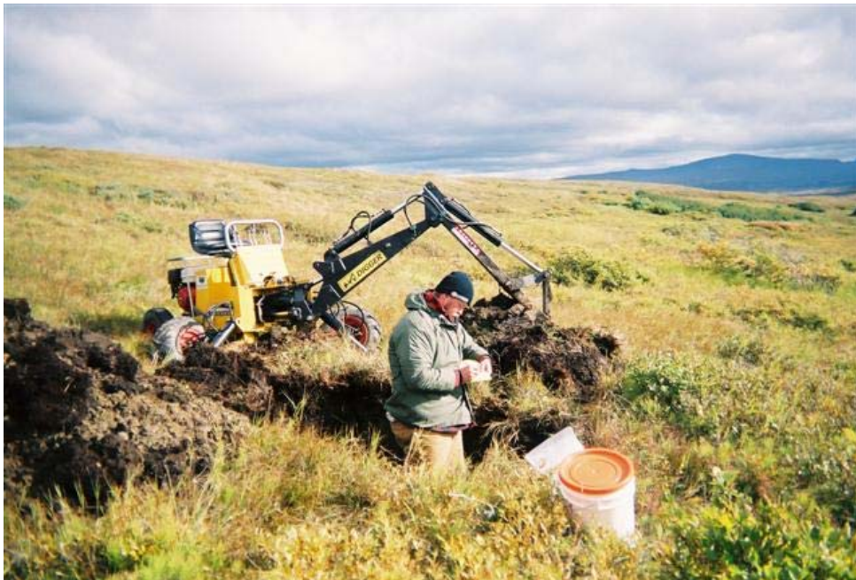
FIGURE 14-14: Geologist investigating a geotechnical test pit. Amy Tomson examined the sidewalls and back dirt for artifacts, stratigraphic differentiation, and any paleontological remains.
