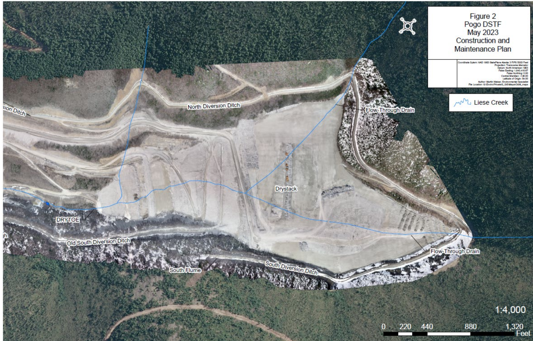
Figure 2: Flow-Through Drain Locations
