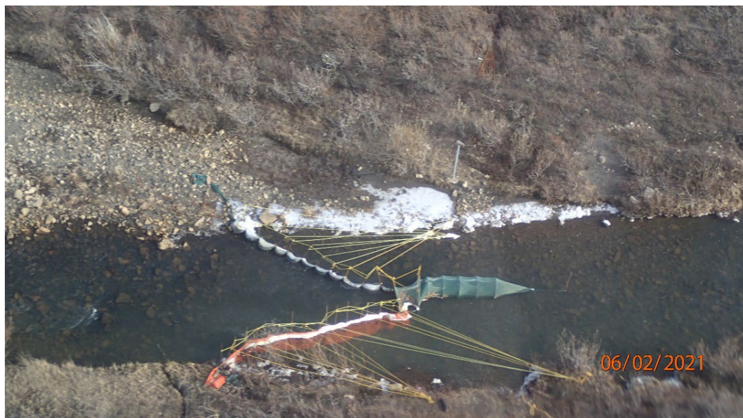
Figure 7. Aerial view of the North Fork Red Dog fyke net on the morning of June 2, 2021. Air temperatures were below freezing the prior night, so ice had formed on the fyke net.
