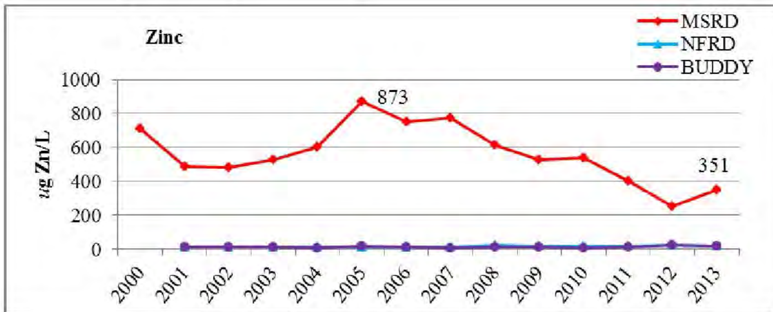
Figure 16. Median Zn concentrations in Mainstem Red Dog, North Fork Red Dog, and Buddy Creeks (2000 to 2013).
