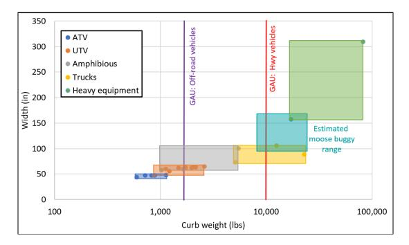
**Figure 1.** Typical widths and weights of different types of vehicles used in the Fortymile area.
