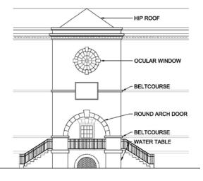
The defining features of the Renaissance Revival style is shown in the tower elevation drawing of the Augusta Arsenal.
