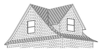
An example of a cross-gable roof and continuous wall shingles.
